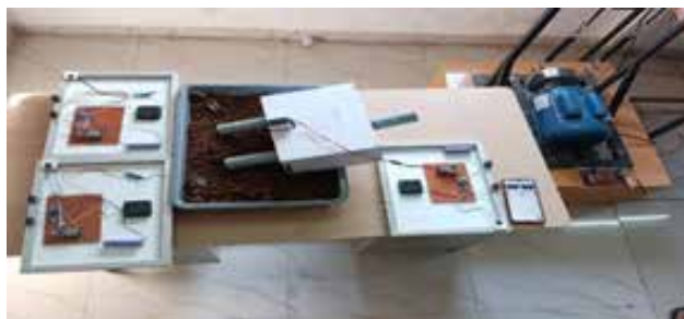
Fig. 15 Water Management and Pump Control System
